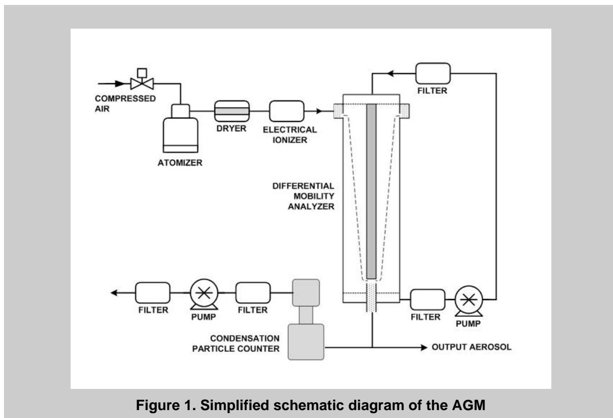
**Figure 1. Simplified schematic diagram of the AGM**
