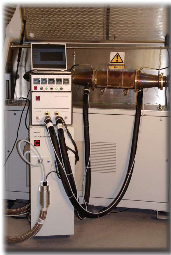
DMS500 with Dual Sampling Accessory sampling from DPF Testing System
