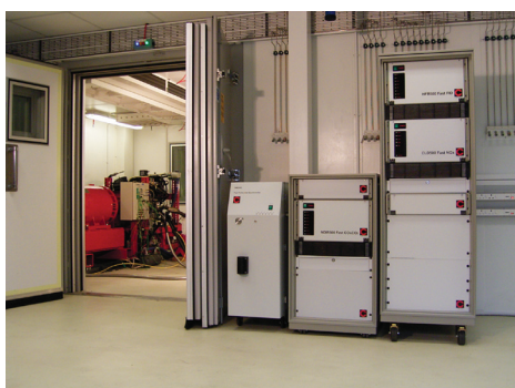
DMS500 shown with other ultra-fast Cambustion analyzers (HC, NO x , CO & CO 2 )
