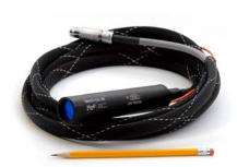
The miniLDV probe, the size of a small flashlight, is self contained and permanently aligned; no calibration required by the user. The probe contains a laser, miniature beam shaping optics, receiving and detection optics.
