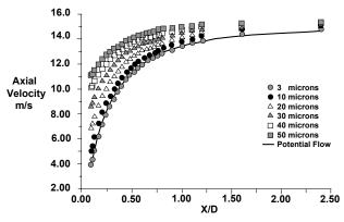
Figure 8. Particle response to the stagnating flow impinging on a right curricular cylinder. The free-stream turbulence intensity was approximately 30%.
