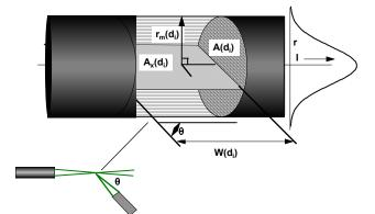
Figure 6. Schematic diagram of the sample volume showing the focused beam diameter, the apparent fringes formed by the intersection of the two laser beams, and the limitation of the length of the beam by the image of the slit aperture located in the receiver optics package.
