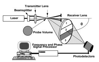
Figure 5. Schematic diagram of the PDPA showing the segmented receiver that collects light from three different apertures at known separation.
