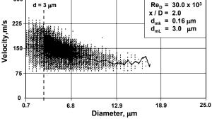
Figure 10. Plot of the drop size versus the drop velocity with each point on the plot representing a single drop measurement. The particles larger than 3 mm begin to lag the high velocity turbulent flow excursions.
