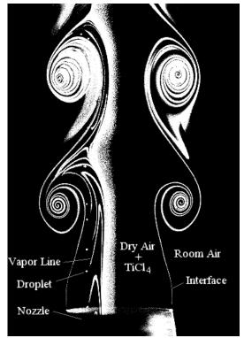
Figure 4. Phase-Locked images of the droplets and vapor lines along with the jet/air interface.
