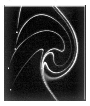
Figure 2a. Weak interaction shows a small deflection of the drops and an accumulation of the small sub-inertial particles in the core of the eddy.
