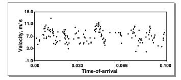
Figure 13. Measured velocity for the particle arrivals with each dot indicating a single particle. The groups of drops indicate clusters.
