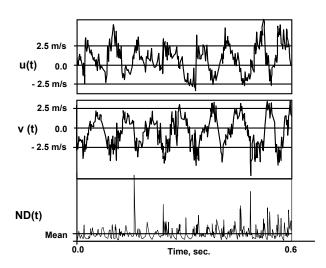
Figure 15a. Raw data for the stream-wise and crossstream velocity versus time showing the shedding frequency with the superimposed turbulence fluctuations. The lower frame shows the time dependent number density computed for short uniform time intervals.
