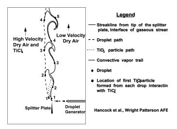
Figure 1. Schematic drawing of the apparatus of Hancock, et al.(1992) for visualizing the interaction of drops with vortices in a shear layer.
