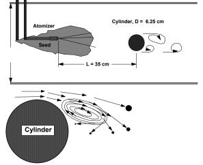
Figure 14. Particle interaction with a vortex street shed by a right circular cylinder. Lower figure shows the expected particle response.
