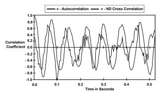
Figure 15b. Velocity versus time plot after the autocorrelation was used to filter the data. The cross-correlation of the time dependent number density with the velocity was computed and displayed.
