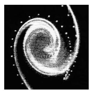
Figure 2b. Strong interaction showing the wrapping up of the drop stream into the vortex to form the streak formation resulting in a high local drop concentration or clustering.
