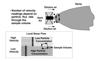
Figure 7b. Schematic showing the possible measurement errors due to particle concentration gradients
