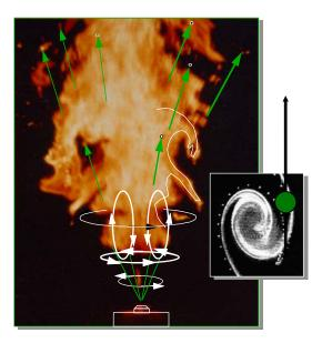
Figure 12. Photo of a spray flame using a pressure atomizer and swirl dilution air to stabilize the flame. Large spray drops injected at high velocity pass through the swirl and recirculation whereas small drops respond to the air flow field.
