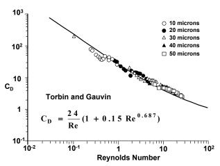
Figure 9. Reduced data of the Drag Coefficient as a function of Reynolds number showing the agreement with the correlation of Torbin and Gauvin.
