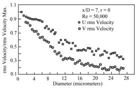
Figure 11. Streamwise and cross-stream turbulence intensity for a turbulent high speed jet measured as a function of particle size.
