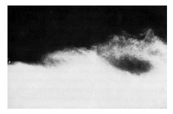
Figure 3. Instantaneous flow visualization showing the dispersion structure for a polydispersion of particles in a forced shear layer (from Lazaro and Lasheras, 1989).
