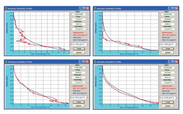
Integrated Water Vapour measurements remain accurate even with LWP of 1000 g/m2.
