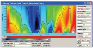
The Simple Zenith Observation Mode shows comparing poorer resolving of the vertical structures in the lower 500 m layer.
