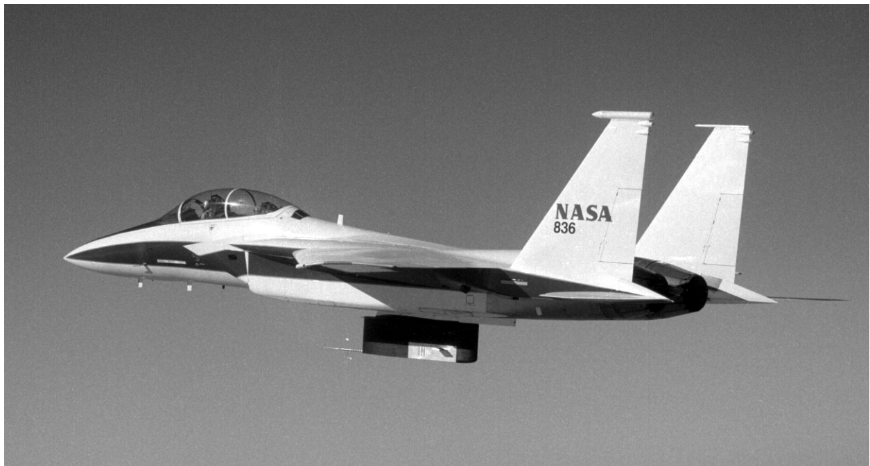
Figure 1. The F15-B in flight with the FTF and test article installed.
