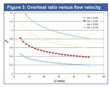
The choice of wire voltage  $V_w$  will depend on the type of measurements to be performed. An important parameter that characterizes the response of hotwires is the wire overheat ratio  $a_w$ , which is defined by:
