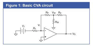
In practice, a hot-wire sensor is connected to the CVA with a BNC cable. Contrary to other types of anemometers, the cable length does not affect the stability of the circuit, so that very long connecting cables can be used. Any type of commercial or self-made hot-wire can be used with the CVA as long as the wire resistance stays in the specified range of  $R_w$ . The output voltage  $V_s$  can be recorded with a stan-
