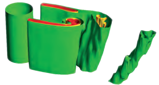
3D Reconstruction: the vorticity field is reconstructed in three-dimensions using a time-resolved phase averaging approach with POD and LDV phase reference signals.
