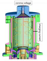
the desired charging (ion) current. Recirculating HEPAfiltered sheath flows prevent particle deposition (including
