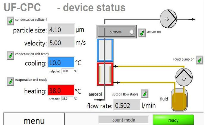
Figure 3: Touch screen user interface showing device status
