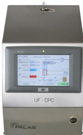
The Palas® condensation particle counter UF-CPC is available in three models, each of them being optimized for a different concentration range. Model 50 is optimized for low concentrations (e.g. after a filter or in an hospital operating room), whereas model 100 is appropriate for medium concentrations (e.g. ambient monitoring). Model 200 offers single particle counting up to 1,000,000 particles/cm<sup>3</sup> (e.g. for printer emission studies).
