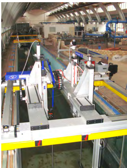
LaVision's stereoscopic 3D underwater PIV system at the Franzius Institute Hannover
