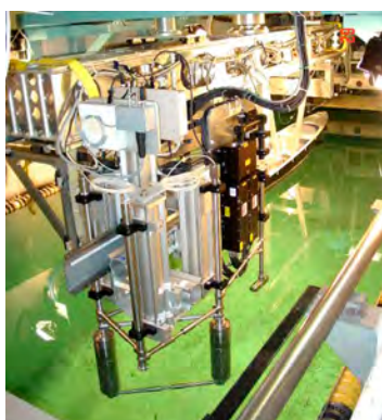
large towing tank facility with submerged PIV system
