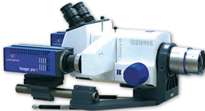
stereoscopic Micro-PIV setup
