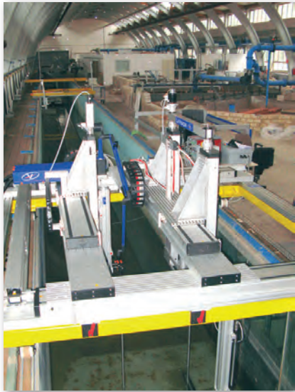
highly modular, stereoscopic 3D underwater PIV system
