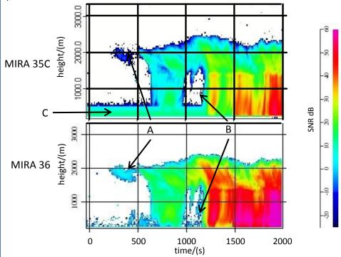
Estimates of the cloud structure are broadly in agreement, although in areas A and B the cloud detection threshold of MIRA 35C is not always reached. The turquoise band below the 400 m level (Area C) is due to the preliminary signal processing of the prototype. Implementing the more sophisticated algorithms of MIRA 35 is planned and will remove this artifact.
