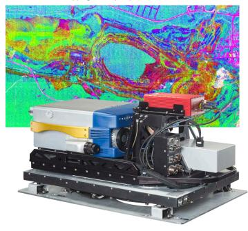
Generate georeferenced hyperspectral maps with the Hyper-Cam Airborne Platform.
