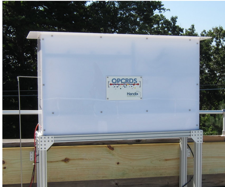
OPCRDS in weatherproof enclosure and custom support stand located on the roof of an air monitoring station in Great Smoky Mountains National Park to study humidity impacts on visibility.
