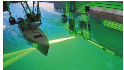
Stereo-PIV system in a towing tank, courtesy G. Jacobi, TU Delft [21]
