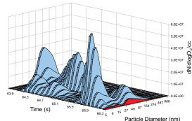
The plot above shows pine smoke sampled with the DMS500 at the full 10Hz data rate. Note that some features of this spectrum last just 200–300 ms; even with a high sampling rate, these subtleties would be blurred out with any instrument with a true response time slower than this.
