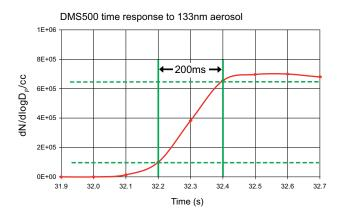
Using Cambustion's long experience in the fluid mechanical design of fast response analysers, the DMS500's response to a step change in concentration ( $T_{10-90\%}$ ) is just ~200 ms, or ~300 ms with a 5 m sample line (1 µm range). By Nyquist's criterion, 200 ms is the minimum response time which can be correctly resolved by an instrument with a 10 Hz sampling rate.
