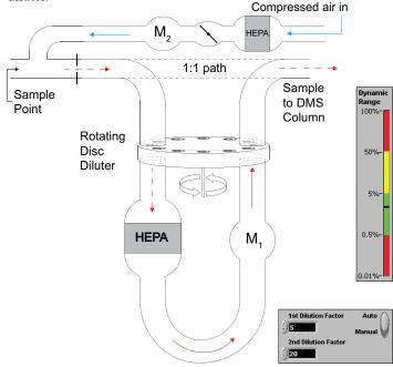
Primary dilution at the point of sampling avoids condensation and agglomeration, and the high ratio secondary diluter allows sampling from a very wide range of aerosol concentrations with over 9 orders of magnitude dynamic range. This single instrument is thus suitable for applications ranging from ambient monitoring to sampling the highly concentrated smoke from pyrotechnic devices or mainstream cigarettes.
