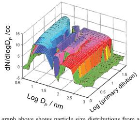
The graph above shows particle size distributions from a flame, into which a solution of  $MgCl_2$  was atomized. The DMS500's primary dilution system was used to provide a flow of nitrogen for dilution and quenching at the sample probe, and the plot shows the size spectrum as a function of this dilution.
