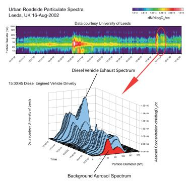
With the best sensitivity amongst real-time particle sizers, the DMS500 *MkII* brings transient capabilities to ambient pollution measurement. The instrument is capable of unattended operation with scheduled sampling and auto-zeroing via its unique built in HEPA filter system, and there is no limit to the length of data files. External devices such as cameras can be triggered when the particle concentration exceeds a preset level. The rapid response
