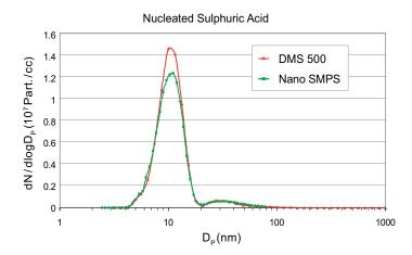
A high sample inlet flow rate (up to 8 slpm) and the unique use of multiple sheath flows in the charging system minimize particle loss by diffusion, even down to 5nm.
