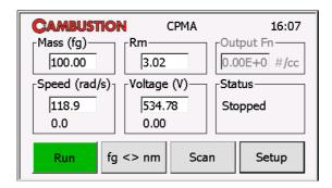
For accurate resolution, the sample flow should be measured and entered. (An optional Aerosol Flowmeter accessory allows this to be automated).
