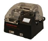
The CPMA is used with an external pre-charger, which may be of the radioactive, X-ray or corona types.
