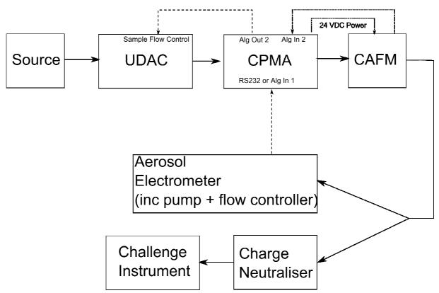
Set the output function of the CPMA to give  $mg/m^3$  from the electrometer. This can then be read off the CPMA display or logged to an Output Function File.
