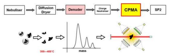
Figure 3: A recommended experimental setup for the mass calibration of the SP2
