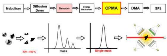
Figure 6: An alternative experimental setup for SP2 mass calibration
