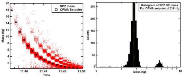
Figure 4: Time series of CPMA setpoints and corresponding SP2 masses for each setpoint
