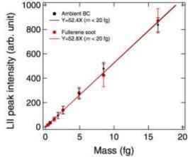
Figure 2: Mass calibration of the SP2 is performed by relating LII peak intensity to particle mass
