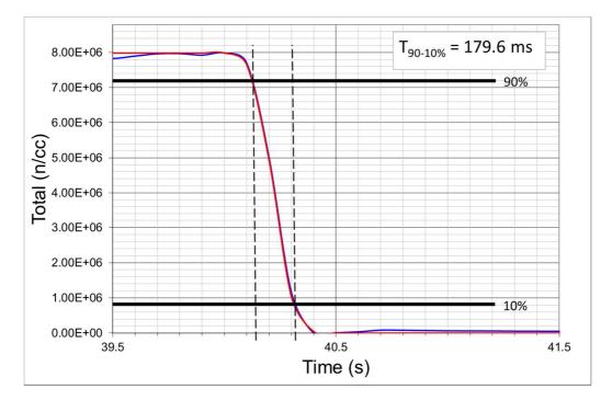
Curve fitting of this data shows that the  $T_{90-10\%}$  response time is 180 ms. Coupled with a data rate of 10Hz (appropriate for the physical response of the detectors) this demonstrates the DMS500's ability to resolve highly transient features.
