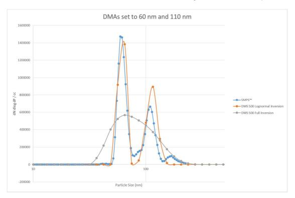
In each case, both the full spectral and bimodal lognormal inversions of the DMS500 are shown. The lognormal inversion is capable of much higher resolution than the full inversion, and the DMA modes are resolved to be almost as narrow as the SMPS can. The full unconstrained inversion does indeed show less resolution than the SMPS, but is still capable of resolving multiple peaks per decade of size range.
