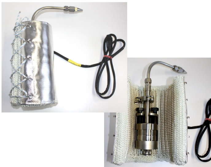
Dekati® PM10 Impactor placed inside a heating jacket to heat the impactor in out-stack measurement setup
