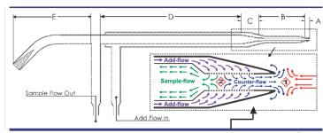
Inset detail shows tip assembly air flows.
