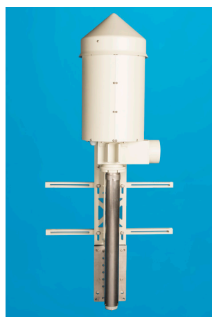
Photo of CVI inlet with wind tunnel assembly installed.
