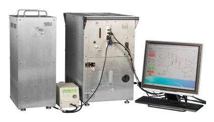
Measure the water uptake by aerosols as large as 2 micron diameter up to 93% RH
