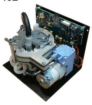
Collect filter sampels for time-resolved aerosol chemistry measurements
