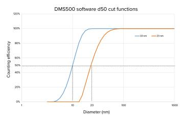
Particle losses are size dependent — measurement of the full size distribution allows automatic correction for transport losses, a correction not possible if only measuring a single concentration.
