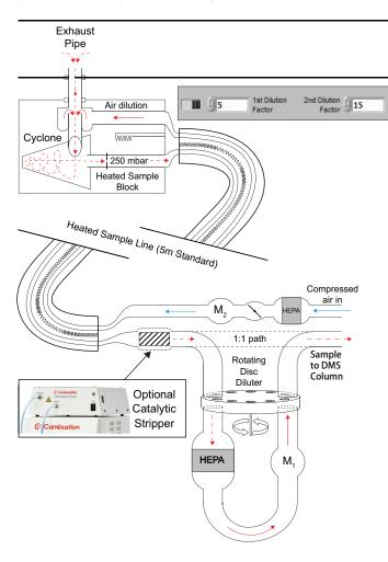
This provides 1st dilution at the point of sampling to avoid condensation and agglomeration, and a user controllable high factor 2nd diluter allows sampling from a very wide range of concentrations.
