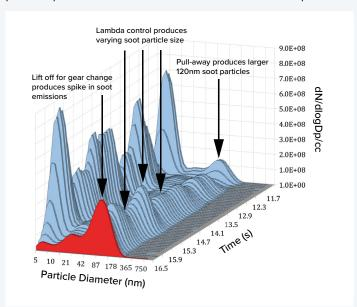
Variations in particle size affect the relationship between PN and PM. Changes in size distribution can also affect the proportion of particles falling within the counting regions for PN (>23nm for Euro 6 and >10nm for Euro 7). Oil consumption effects may be of particular significance for the 10–23nm size range.
