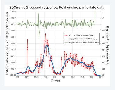
The above graph shows that only with a 300ms  $T_{10.90\%}$  response are the effects of lambda control resolved — the 1.8s  $T_{10.90\%}$  response does not identify important features, despite an identical data sampling rate.
