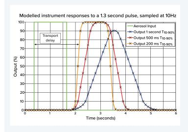
The 1 second  $T_{10-90\%}$  data fails to resolve the true maximum concentration.
