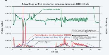
Even when fitted with a Gasoline Particulate Filter, the lower filtration efficiency achieved (due to the difficulty forming a soot cake at higher temperatures in lean conditions) on a spark ignited engine means that optimisation of engine out emissions is crucial as part of emissions compliance.
