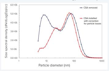
The CSA requires no additional dilution, ensuring measurement sensitivity remains unaffected. The DMS500's fast time response is also not compromised when the CSA is fitted.
