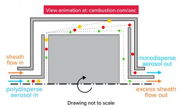
With the classifier stationary, all particles follow the sheath flow, and are lost in an internal HEPA filter.
