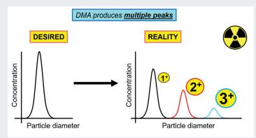
The AAC offers significantly improved transmission compared with the DMA, since the DMA is affected by poor charging efficiency, meaning that only a small fraction of the target particles receive a single charge and make it through the classifier.
